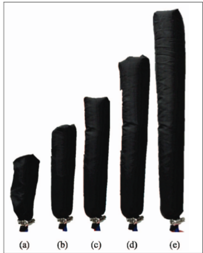
Fig. 14. Extension stages of a fabric-based actuator going from (a) being the least extended, (b)(c)(d) showing intermediate stages (e) being the maximum extension and inflation. In this system the external structure shown in (a) remains stationary while the material needed to extend everts from the centre of the actuator. [25]
