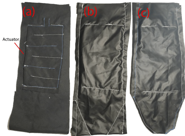
Fig. 15. Image showing the steps to take the fabric section seen in 14 and produce the leg. The fabric square is folded in half along its length, with the actuators facing inwards. A seam is sewn along the edges of the material that curve inwards from either side towards the middle bottom as seen in (b). The excess material is then cut, and the chamber is folded inside out as seen in figure 16.
