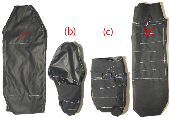
Fig. 16. Diagram showing how the leg is folded inside out after figure 15 from the internal side that the stitch is located on, through the bottom (b)(c), revealing the micro-fibre side (d) with the actuators externally located. The actuators need to be outside the chamber as they are able to provide more contraction by increasing the bending moment through increased distance from the centre. This also increases bending as the contraction has a horizontal component as well as a vertical one, while contraction internally would act primarily by shortening the fabric through a force parallel to the length.
